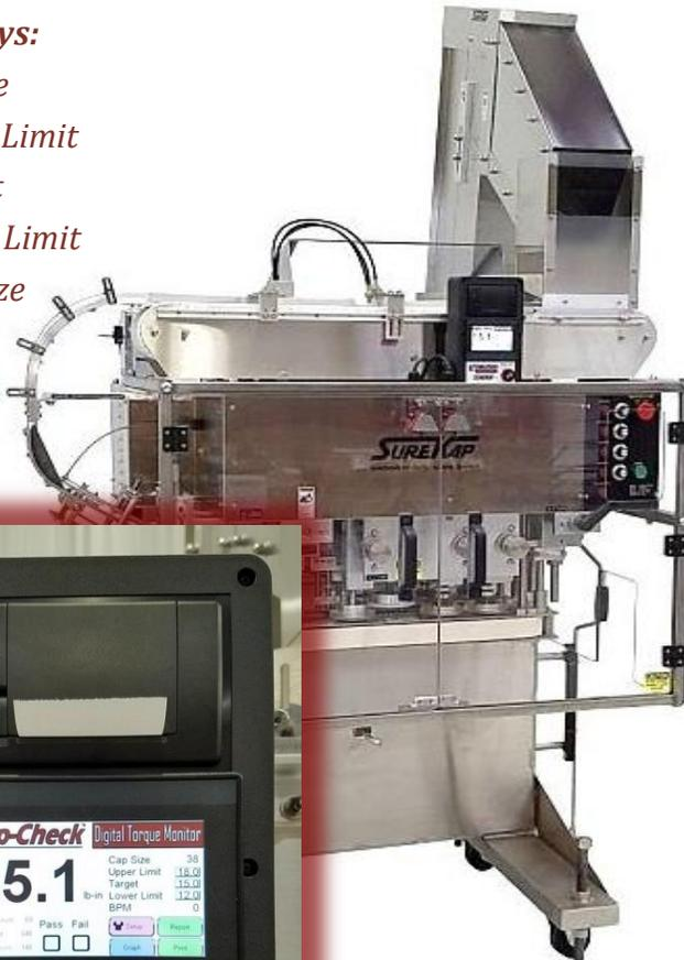
The **Kap-Check**™ Model KC15 Digital Torque Monitor is a fully automatic, PLC controlled, inline, torque measuring system. This unit is a perfect option for your new SureKap Capper or it can easily be added to your existing SureKap Capper or Retorquer.
